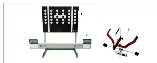
Fig. 3. The stand for tests of the setting and calibration of cameras for the control of the driving path.
