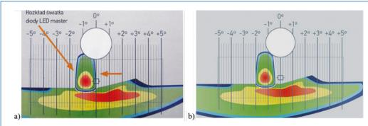
Fig. 2. Control of light distribution of the LED master in LED reflector Matrix. a) location of the field illuminated by the master diode – correct, b) incorrect [11]
