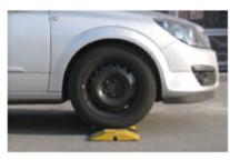
Fig 4. Investigating of the condition of shock absorbers using a body acceleration sensor. Vibration recording with a PTI tester [8]
